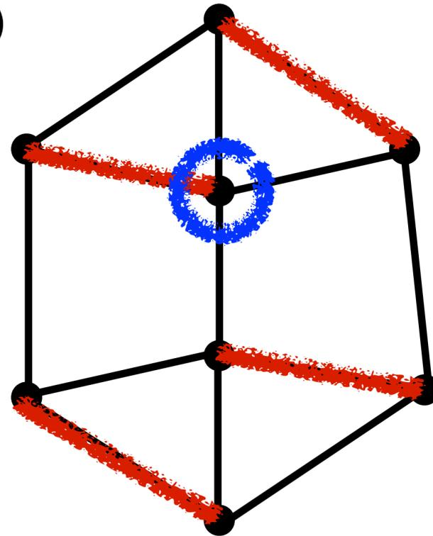
$$\begin{aligned} & \max \sum_{e \in E} x_e \\ \forall v \in V : & \sum_{e \in \delta(v)} x_e \leq 1 \\ & x_e \in \{0, 1\} \end{aligned}$$
