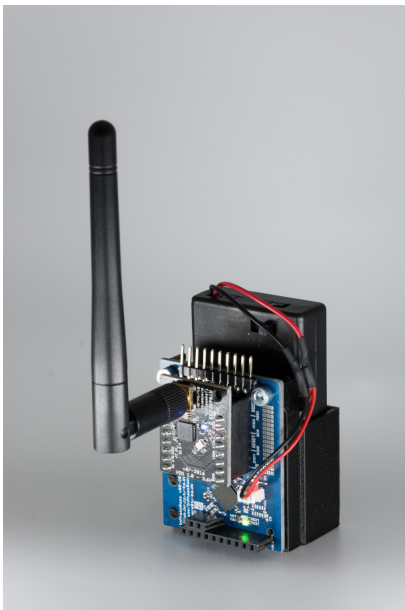
Fig. 3. Battery-powered InPhase sensor node (reproduced from [5]).
