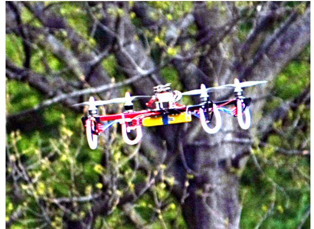
Fig. 4. The flying WSN-based quadrotor.
