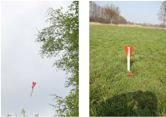
(a) Tree landing (b) Parachute ejection fail
