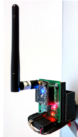
Figure 1: Modular sensor node with AT86RF233 radio module mounted to a wall.
