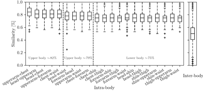
Fig. 4. Similarity of gait-based fingerprints extracted from body locations of the same (intra-body) and different users (inter-body). The results are obtained from Mannheim dataset [9]
