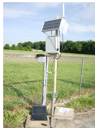
Figure 2: Current solar powered node design with 16W panel
