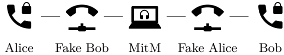
(b) Active MitM: The attacker maintains two separate calls to Alice and Bob and connects the streams.
