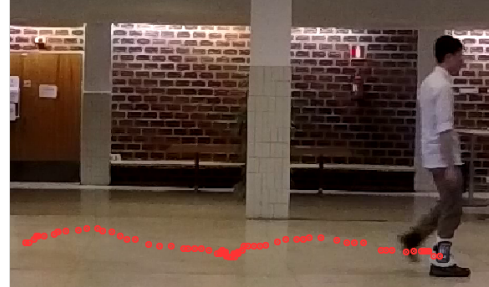
(b) Tracking the z-axis acceleration by manually annotated video recordings (90 fps).
