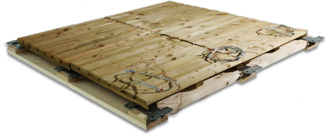
Figure 3. Construction with floor tiles and load sensors.
